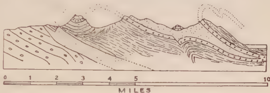
FIG. 353.—The slopes of the sides of the mountains are determined largely by the dip of the rock forming them.
